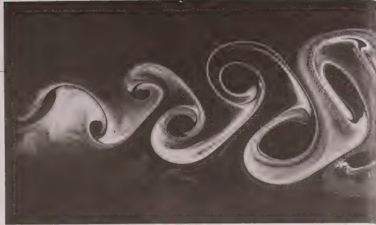
Trains of vortices arise if a solid object is drawn in a straight line through stationary liquid.
